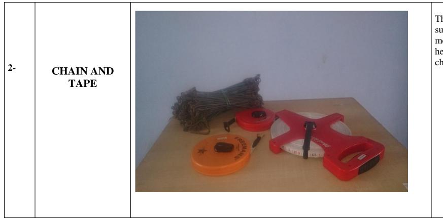
The length of the survey lines are measured with the help of tape or chain.
