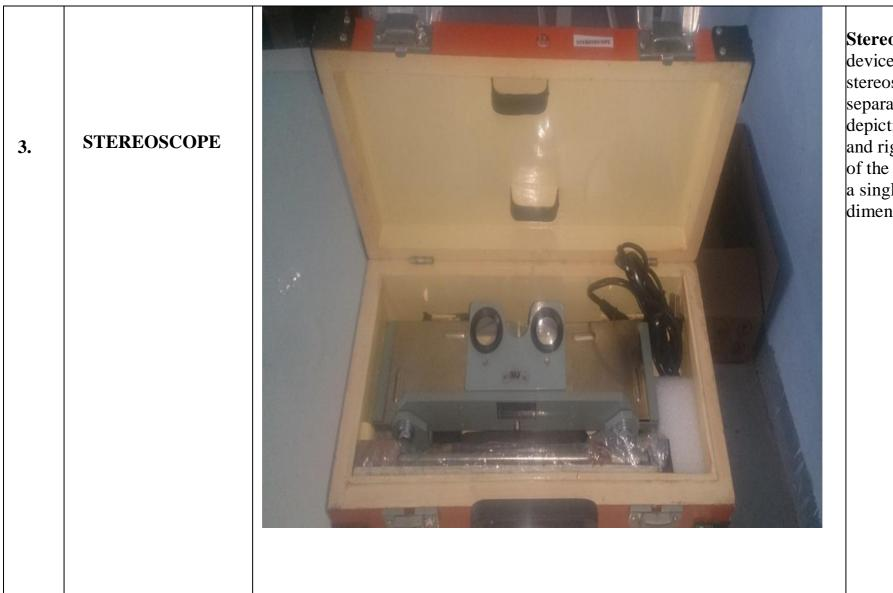
**Stereoscope** is a device for viewing a stereoscopic pair of separate images, depicting left-eye and right-eye views of the same scene, as a single three-dimensional image.
