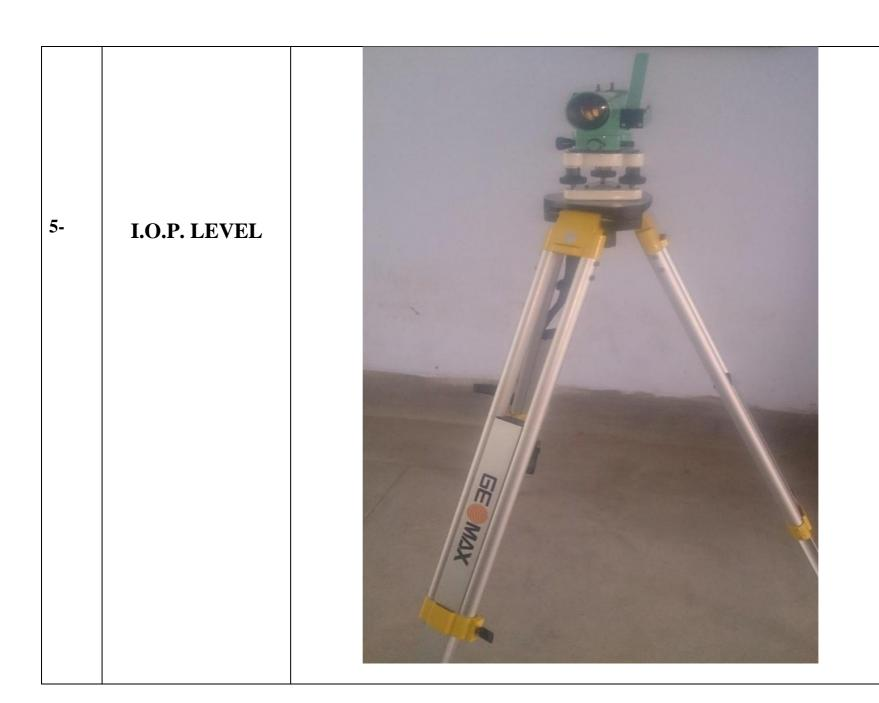
An I.O.P level is an optical instrument used to establish or check points in the horizontal same plane. It is used in and surveying with building vertical staff height measure differences and so transfer, measure and set heights.
