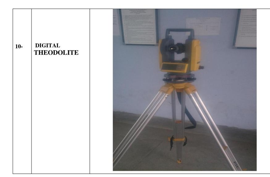
Digital Theodolites serve as a vital surveying instrument and are widely used surveying for the measurement of horizontal and vertical angles. Theodolites also determine the relative location, and are extremely useful in navigation and meteorology.
