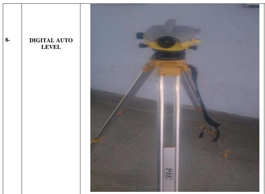
Digital levels improve standards for levelling on sites construction and general surveying tasks. They are simple to use, take measurements quickly, and minimize human error, while the integrated programs enhance levelling work.
