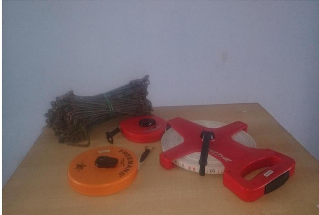
The length of the survey lines are measured with the help of tape or chain.
