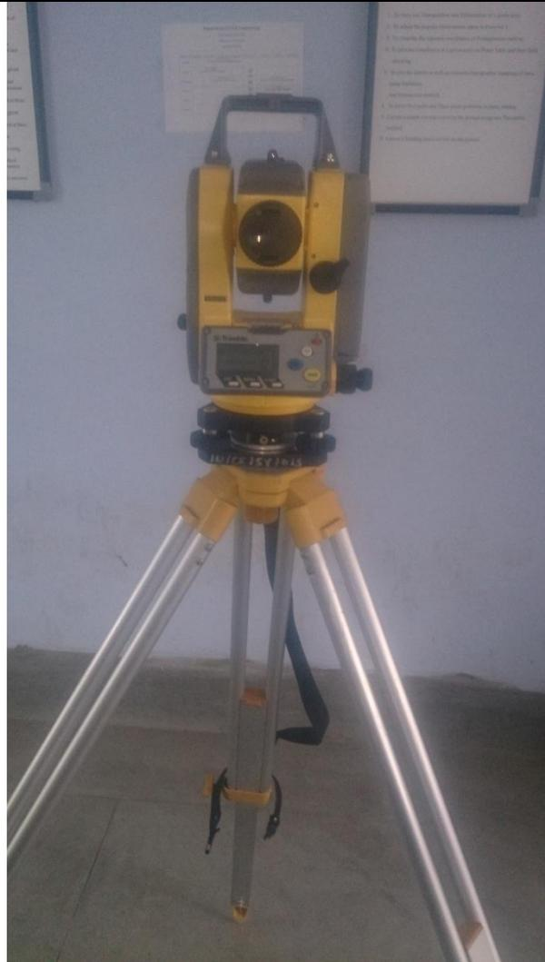
Total station is a combination of **Electromagnetic Distance Measuring Instrument** and electronic theodolite. It is also integrated with microprocessor, electronic data collector and storage system. The instrument can be used to measure horizontal and vertical angles as well as sloping distance of object to the instrument. Microprocessor unit processes the data collected to compute:
