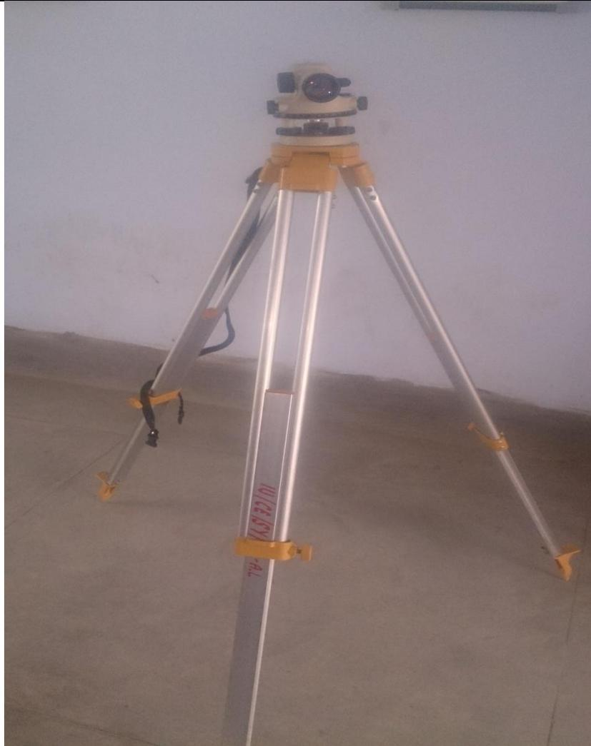
A **auto level** is an optical instrument used to establish or check points in the same horizontal plane. It is used in surveying and building with a vertical staff to measure height differences and so transfer, measure and set heights.
