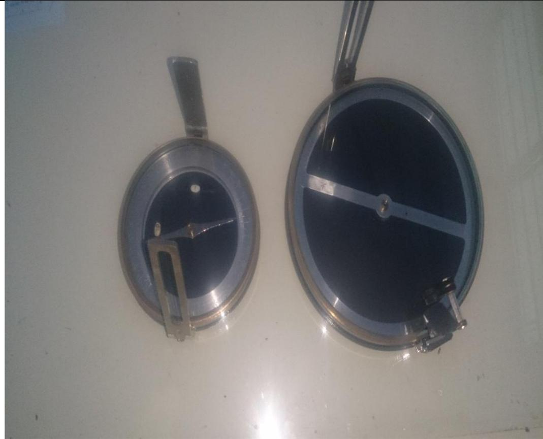
Compass surveying is a type of surveying in which the directions of surveying lines are determined with a magnetic compass. The compass is generally used to run a traverse line. The compass calculates bearings of lines with respect to magnetic north. The included angles can then be calculated using suitable formulas in case of clockwise and anti-clockwise traverse respectively.
