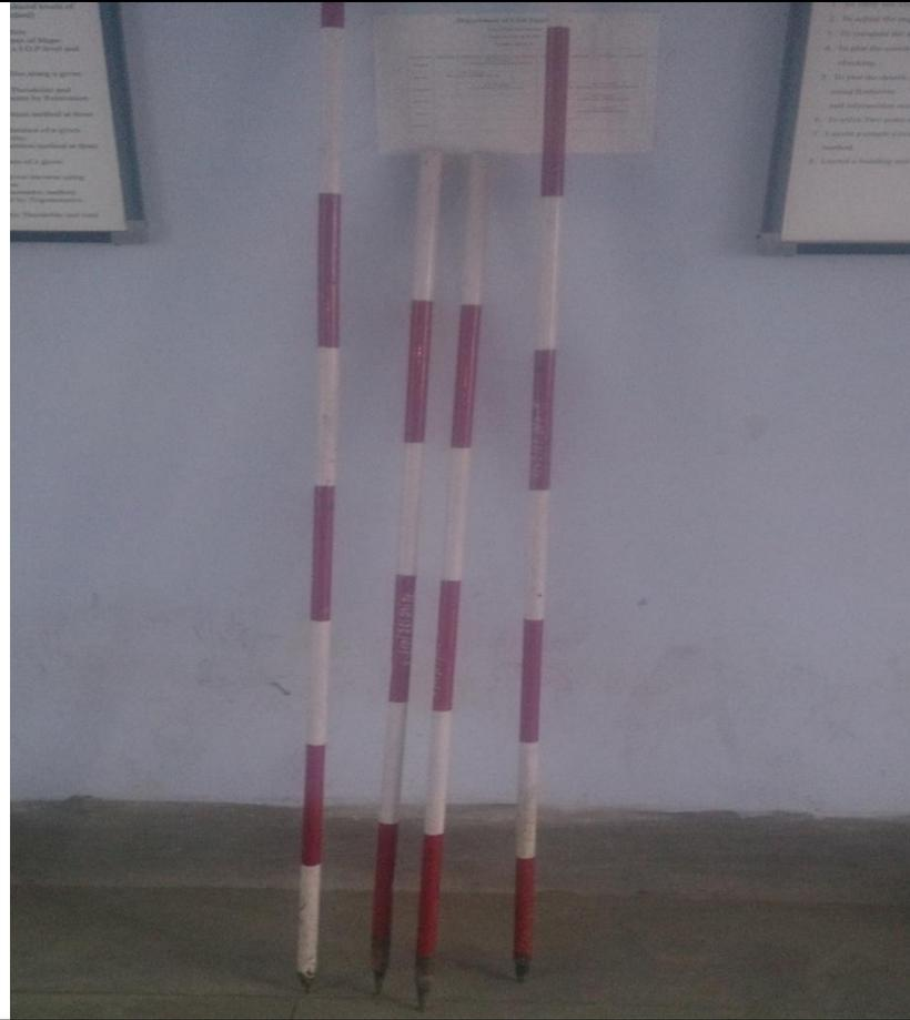
**Ranging rod** is an surveying instrument used for marking the position of stations and for sightings of those stations as well as for ranging the straight lines. Now a days these are made of metallic materials only. These are usually 3 cm in diameter and 2 m or 3 m long.
