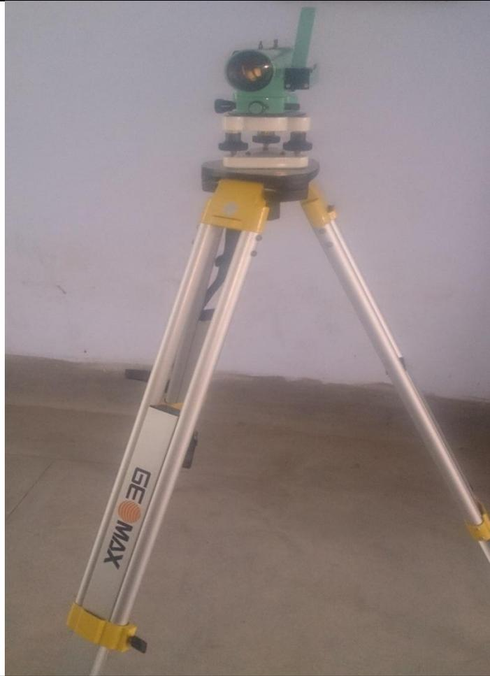
An **I.O.P level** is an optical instrument used to establish or check points in the same horizontal plane. It is used in surveying and building with a vertical staff to measure height differences and so transfer, measure and set heights.
