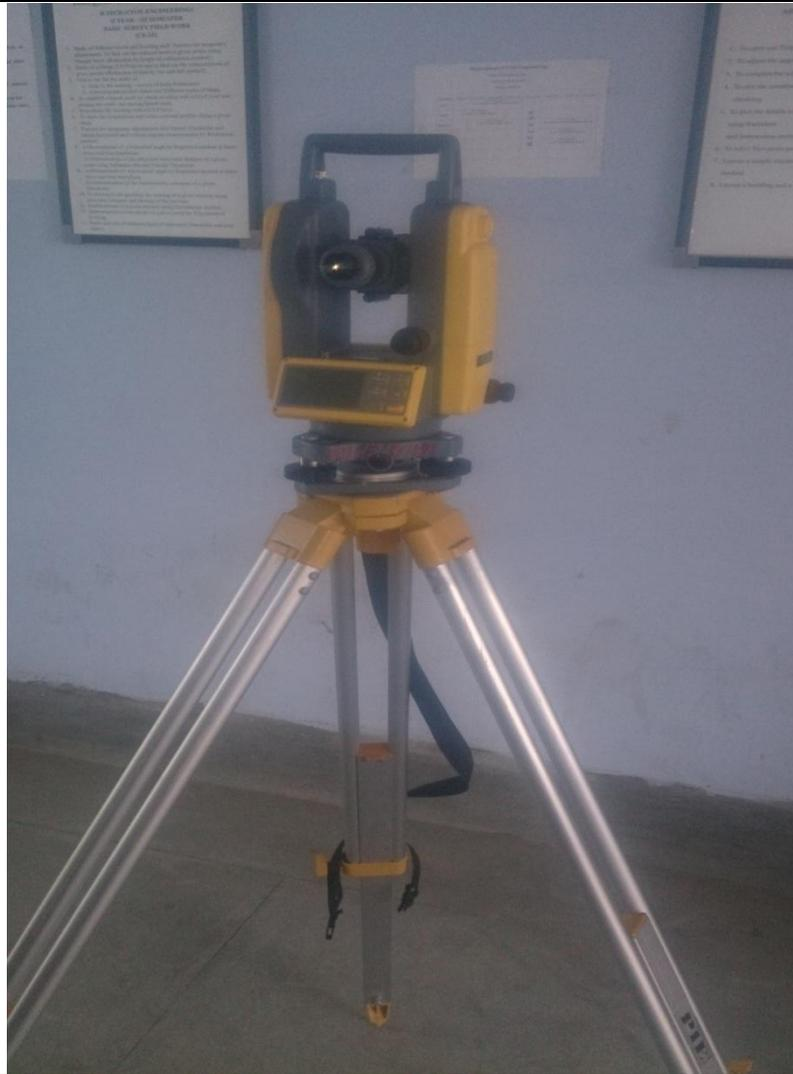
Digital Theodolites serve as a vital surveying instrument and are widely used in surveying for the measurement of horizontal and vertical angles. Theodolites also determine the relative location, and are extremely useful in navigation and meteorology.
