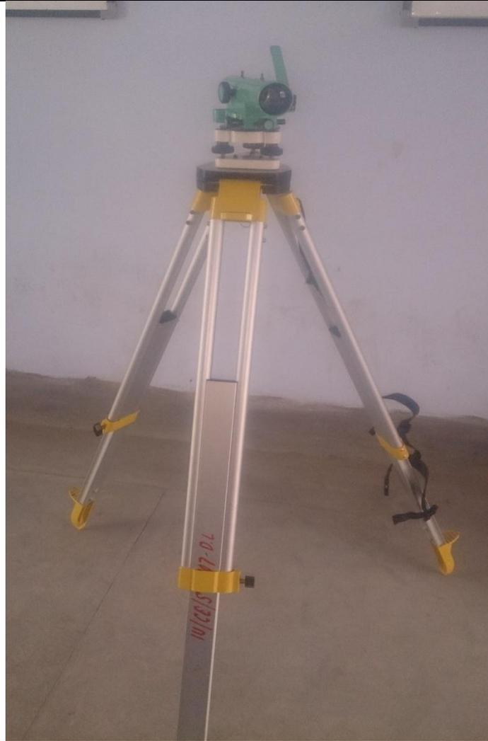
A **dumpy level** is an optical instrument used to establish or check points in the same horizontal plane. It is used in surveying and building with a vertical staff to measure height differences and so transfer, measure and set heights.
