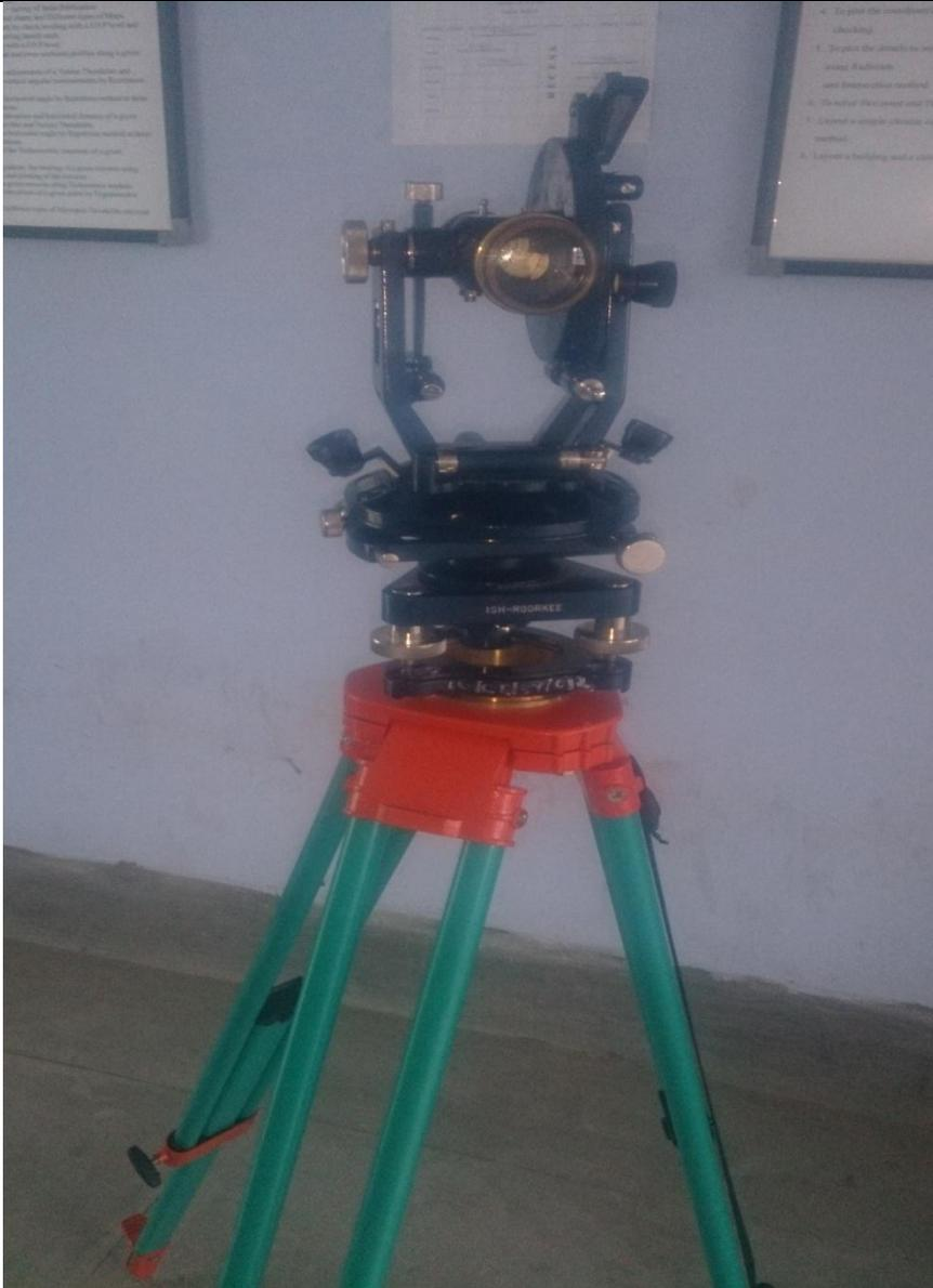
The Vernier Theodolite is also known as a transit. In a transit theodolite . A **theodolite** is a precision instrument for measuring angles in the horizontal and vertical planes.
