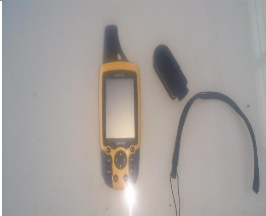
GPS was rapidly adapted for surveying, as it can give a position (Latitude, Longitude and Height) directly, without the need to measure angles and distances between intermediate points. Survey control could now be established almost anywhere and it was only necessary to have a clear view of the sky so the signal from the GPS satellites could be received clearly.
