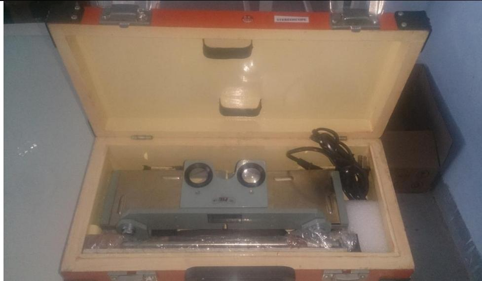
**Stereoscope** is a device for viewing a stereoscopic pair of separate images, depicting left-eye and right-eye views of the same scene, as a single three-dimensional image.
